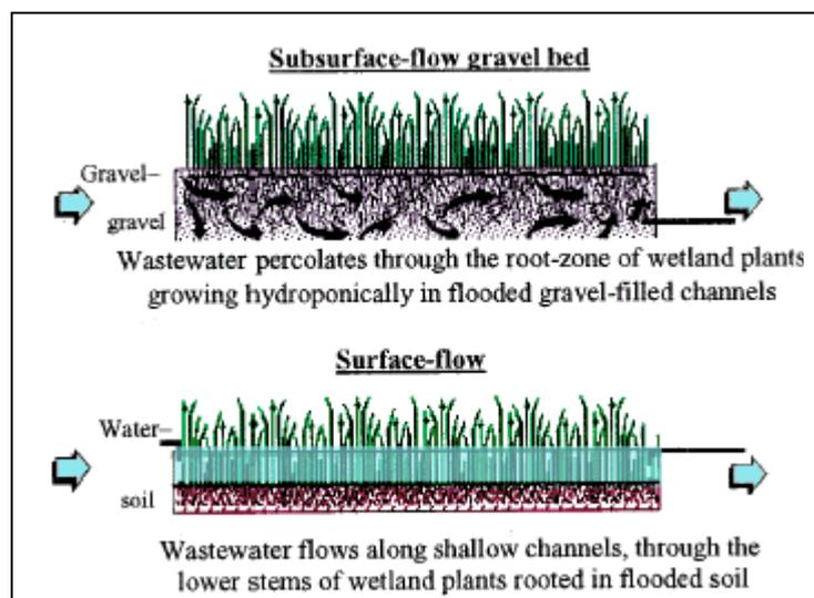
In CW effluents/ polluted waters are channelled into a series of man-made ponds with an impermeable synthetic liner or clay base, filled with either the original soil from the site or with selected substrates (normally sands and gravels). These are planted with vascular hydrophytes, aquatic plants, which quickly develop extensive submerged root systems.
