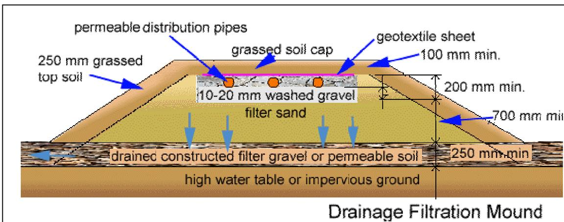
To provide venting of the distribution pipes the pipes may be extended above the mound.
