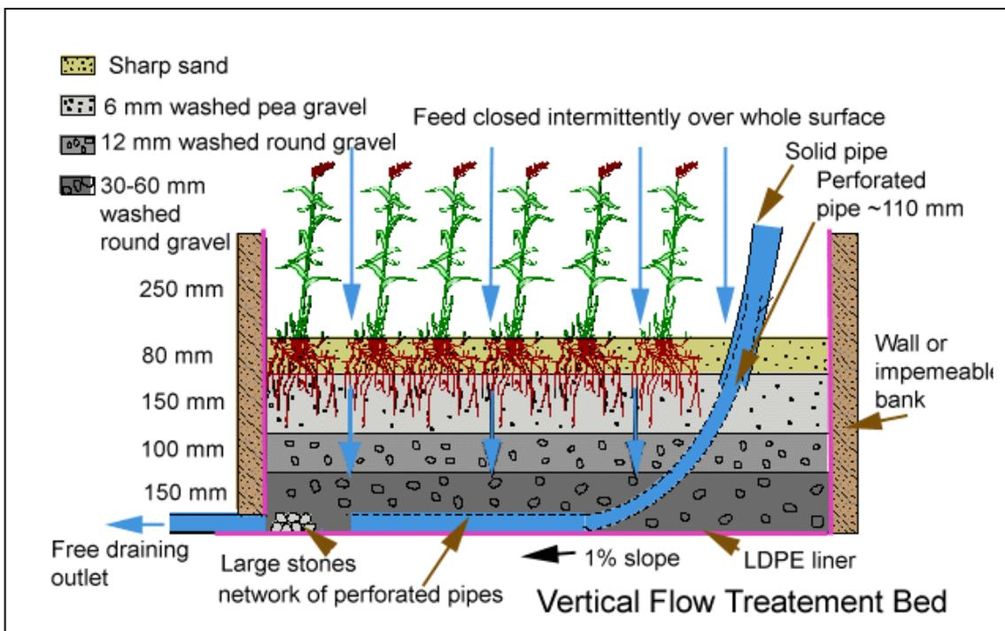
down slope outlet. The overall fall is normally between 1 and 2 metres across the length of the bed. The intermittent nature permits a rest period, for this reason two or more beds are used in rotation.
