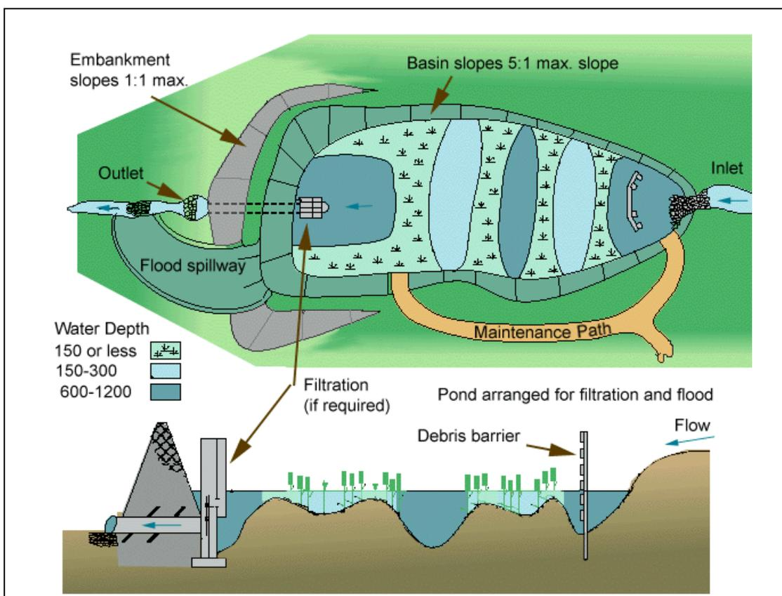
Treatment beds should be protected from inflow of water which may cause flooding and spill from the wetland permitting contaminated water entering the local hydraulic system.
