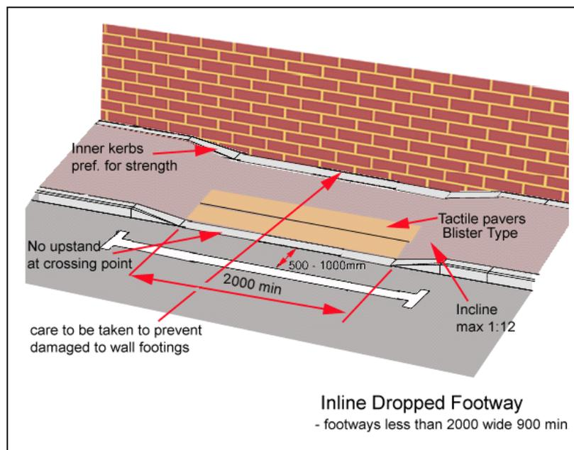
The correct tactile pavers should be used to indicate the crossing. These must only be used where there is a dropped kerb on both sides of the carriageway.
