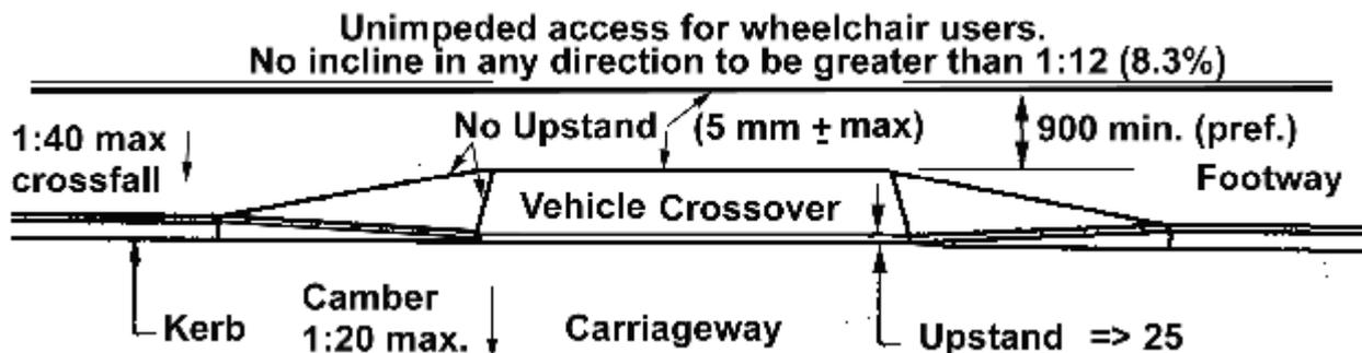
Care must be taken when installing pedestrian flush dropped kerbs and vehicle crossing dropped kerbs that no slope on inclines becomes greater than 1:12 (8.3%). Builders often forget that if they remove and replace one kerb stone and replace it with an angle cut kerb that this angle must be added or subtracted from the existing angle of the footway incline to maintain the correct slopes.
