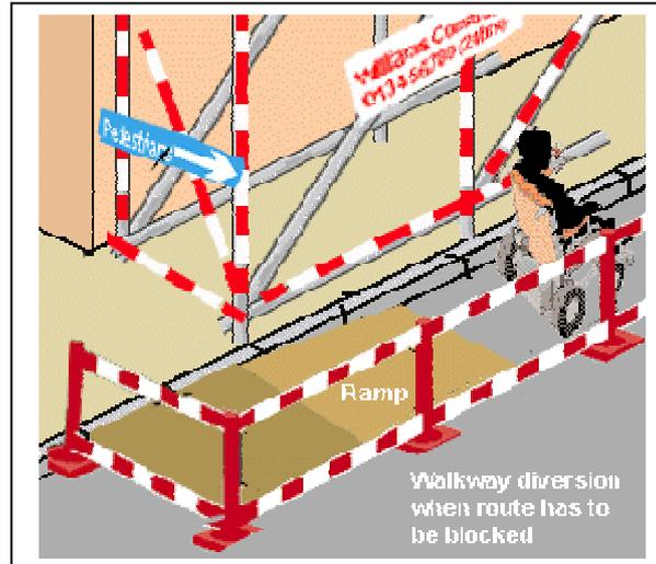
Where the minimum's cannot be maintained a safe diversion should be provided either by using a temporary ramped bypass onto the carriageway, or by placing signs at the closest safe dropped kerb crossing before the obstruction.
