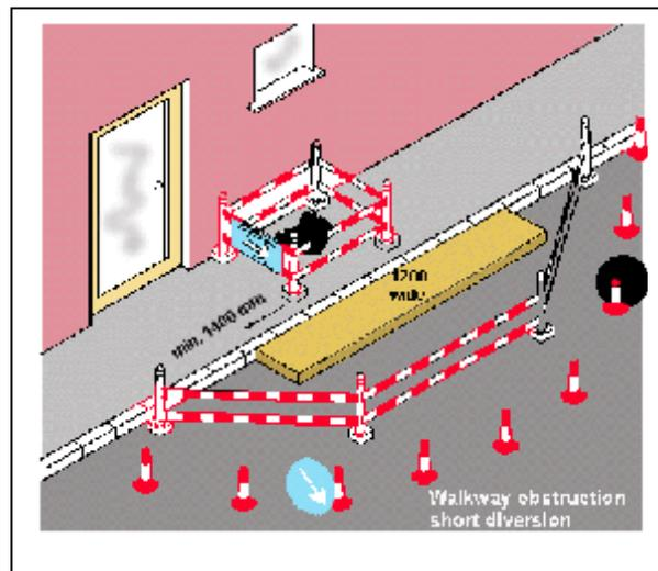
Debris must be kept clear of walkway and carriageway surfaces at all times.
