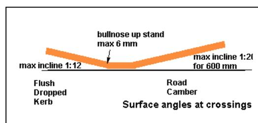
High angle of incidence with road cambers causes puddling and can cause the machine to bottom and stall.
