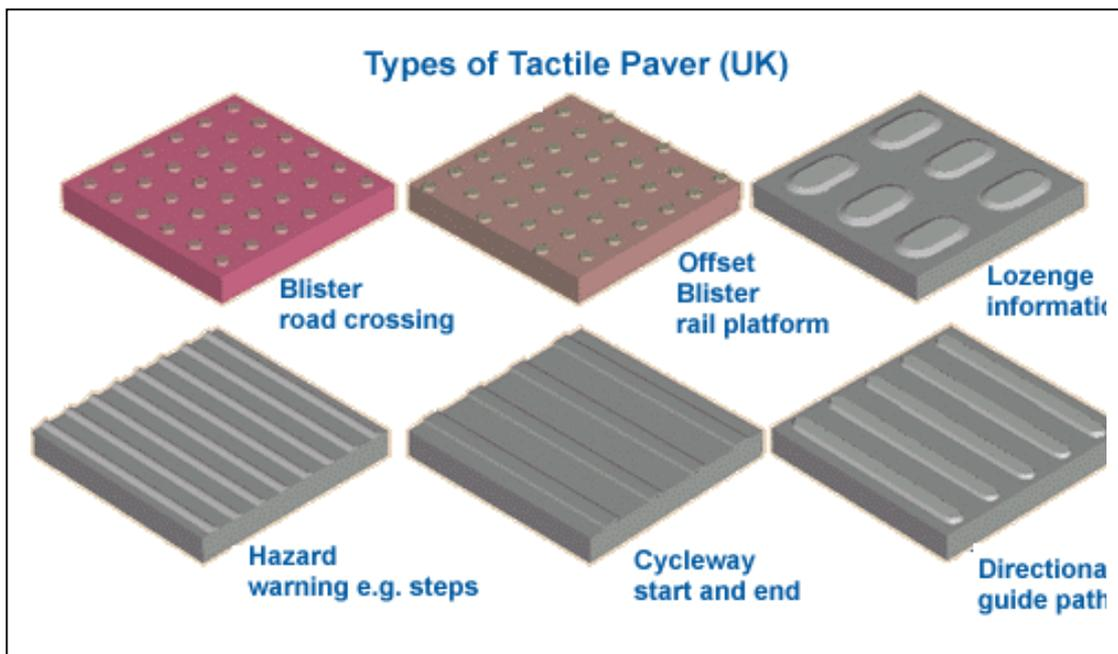
The lozenge paver is used for on street light rail platforms. A single or pair of lozenge pavers are sometimes used to indicate where notices, tactile text or Braille signs are located. This is used to ensure that there is no confusion with kerbs and steps which have lower risers.
