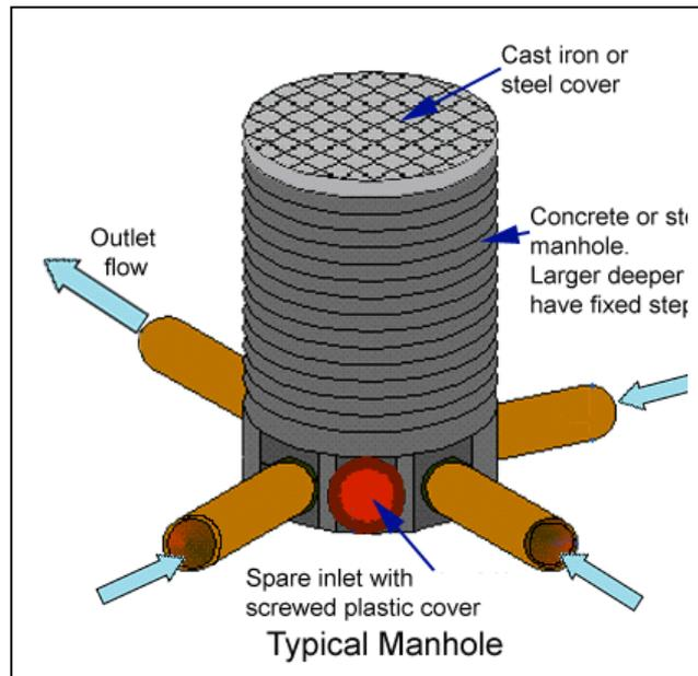
Additional new drainage can be connected to the system via one of these inlets provided that the inlet is the same size or larger than the pipework to be connected. Excavating outside the chamber will expose the stopper cap, which is then removed and the new pipework connected in its place.
