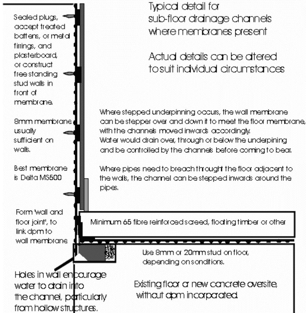
This system can be effective in situations where personnel or damp sensitive equipment or materials are in the room. It can be expensive to use as new floors are required.
