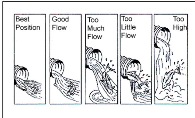
than the jump height local sedentary fish can handle. The best solution has the outlet below the surface of the lower stream.
