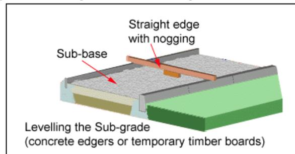
The using a straight edge with a 'nogging' set at the correct distance a quick check of any irregularities can be made.
