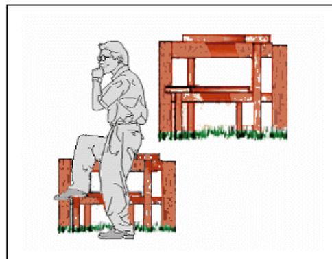
and viewing points and fishing stations. Perches should be maintained and strong enough to support expected weights, 200 x 100 verticals, 73 x 100 horizontals or 300 x 25 thick planks.
